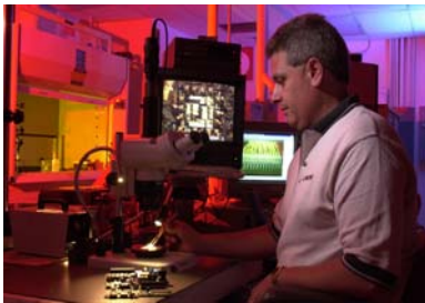
Stereo Microscope with Digital Photography, 1250 times magnification capability
